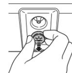
2. Change the air filter. Remove the old air filter with a sharp object and insert the new air filter.
