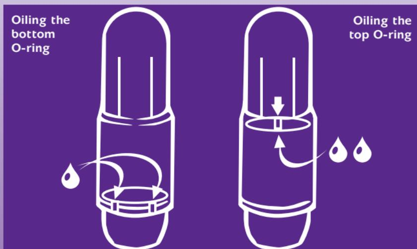
Do not damage or scratch any of the sealing surfaces since this will drastically reduce the pump efficiency.
